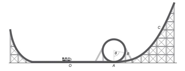
The loop section is modelled by considering the track to be a vertical circle of radius 10 m and the car as a particle of mass mkg moving on the inside surface of the circular loop. You may assume that the track is smooth.
